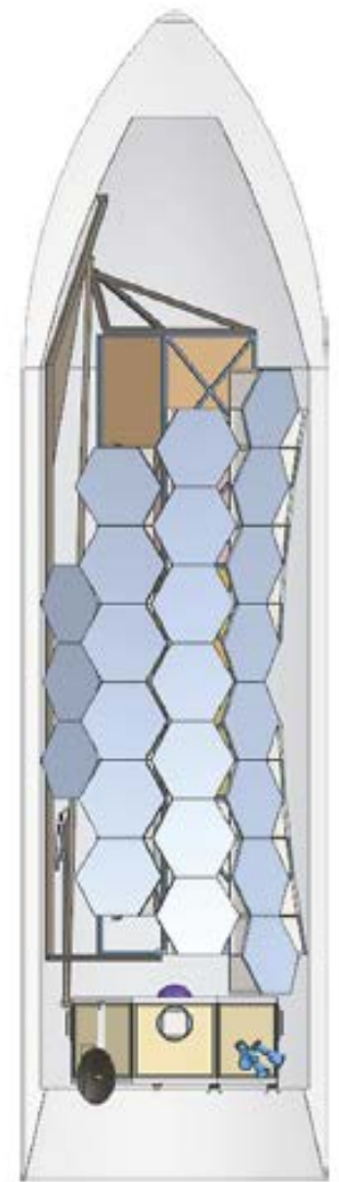
Figure 5-2: A folded 11 m primary mirror, constructed with 54 1.3 m segments, is shown inside a Delta 4-H shroud.
